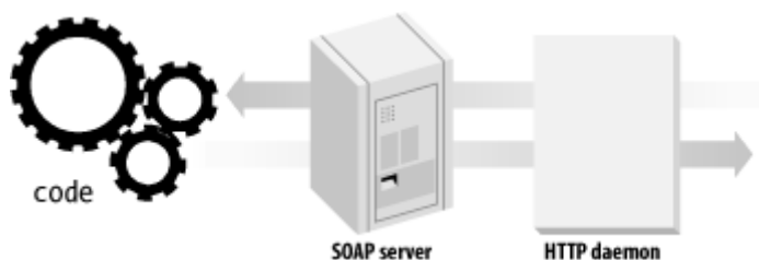
Figure 1. The HTTP daemon passes the request to the SOAP proxy, which then invokes the code behind the web service
